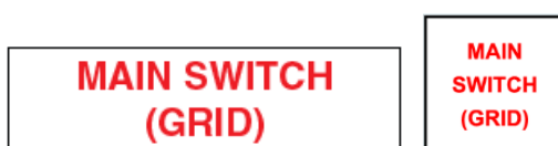
Figure 2: Compliant examples of “MAIN SWITCH (GRID)” labels.
