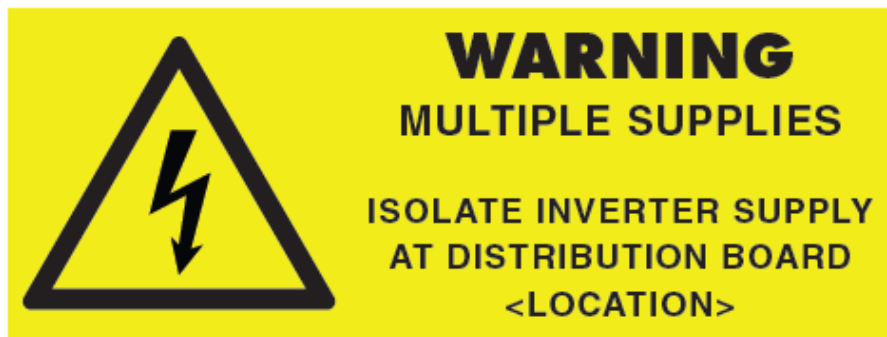
Figure 2: Example of a compliant sign for a main switchboard or distribution switchboards when the IES is connected to a subsequent distribution switchboard. Location information to be included at time of installation.
